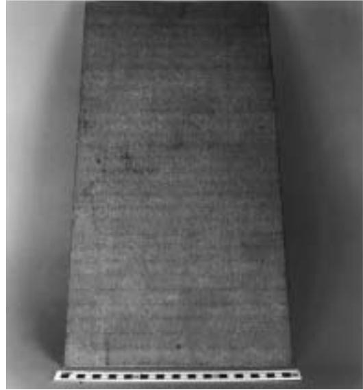
10d Asbestos cement roofing slate.
