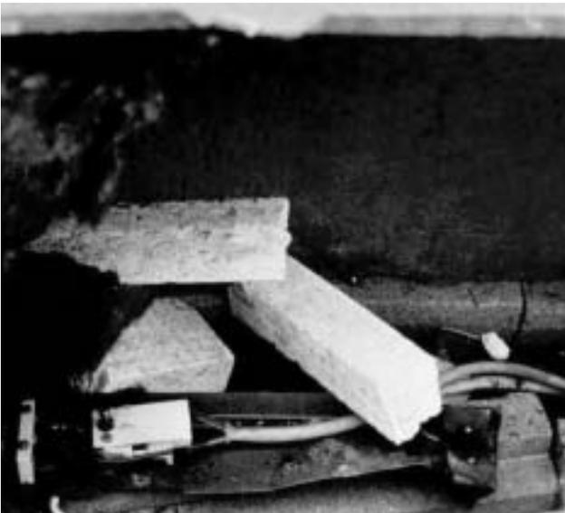
18b 'Caposil' insulation from inside an old electric storage radiator.
