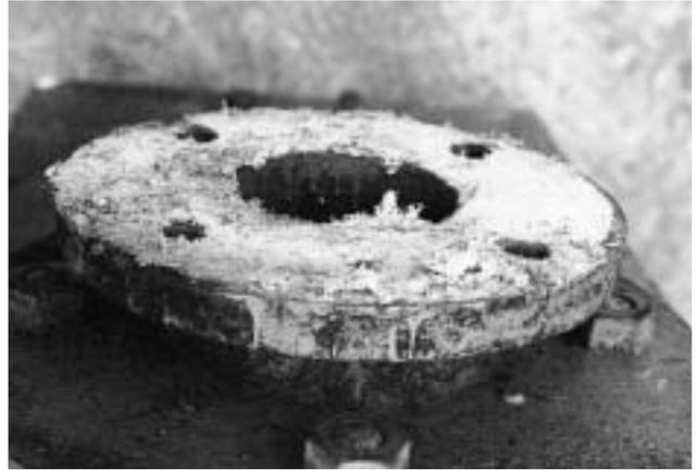
9c Gasket material adhering to a pipe flange.
