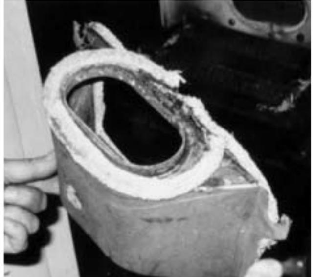
8d Asbestos rope seal in a domestic gas boiler.
