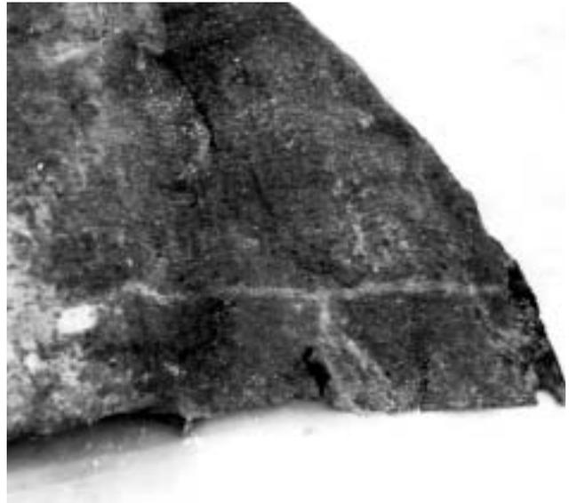
13a Weathered asbestos-containing roofing felt (less weathered material is black).
