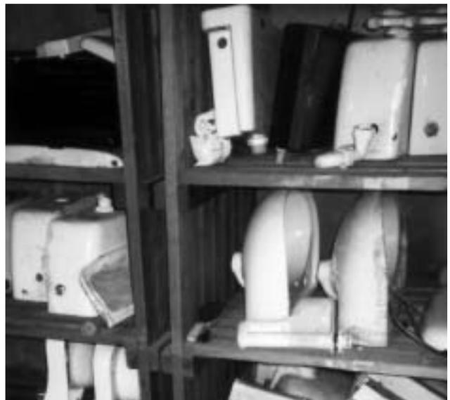
15a Asbestos-reinforced plastic toilet cistern.
